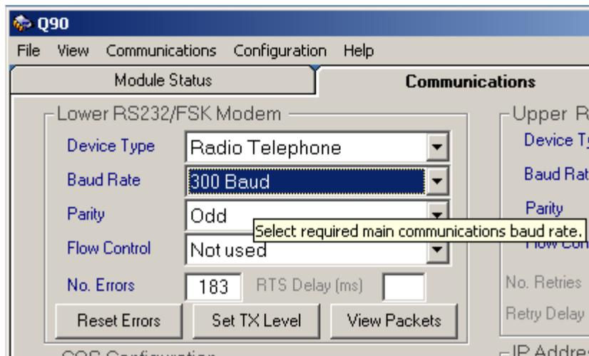
After the appropriate baud rate has been selected, the last thing that needs to be done is to adjust the transmit audio level out of the RTU. This is necessary because the two different types of modem chips have different gain characteristics.
