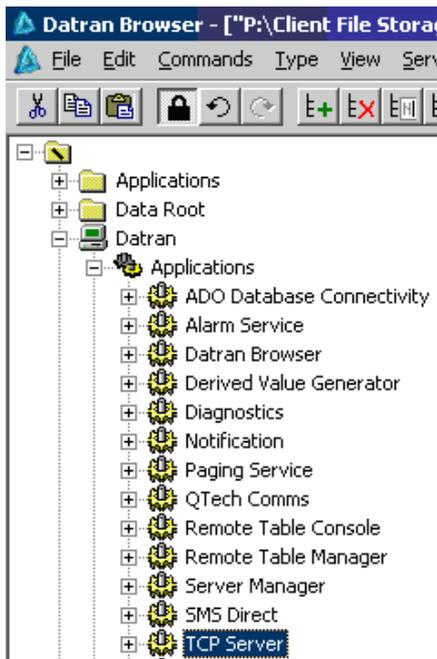
5. Double click "TCP Server". TCP Server is the DATRAN service that manages Supervisor connections and other TCP communications. Click the "State" tab at the top and this shows the current license in the field labelled "Security key".
