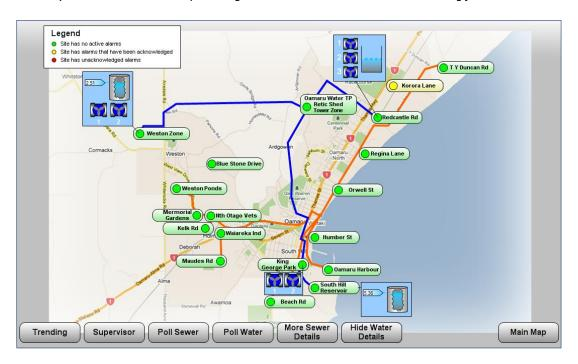
These resources can reside in a typical factory or plant environment or in remote locations. Where the monitored stations are remote, telemetry communication (via radio, land line, cellular link) is used to transport data back to the base station. Telemetry communication is used where direct serial communications with devices is not practicable.
